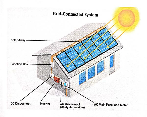
Electric energy or electricity can be produced directly from solar energy by means of photovoltaic cells. The photovoltaic cell is an energy conversion device which is used to convert photons of sunlight directly into electricity. It is made of semi conductors which
