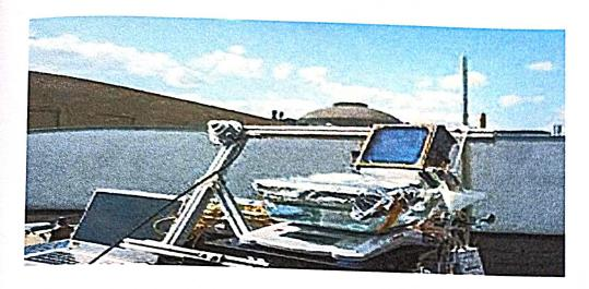
In arid semi and or coastal areas there is scarcity of potable water. The abundant sunlight in these areas can be used for converting saline water into potable distilled water by the method of solar distillation. In this method, solar radiation is admitted through a transparent air tight glass cover into a shallow blackened basin containing saline water.
