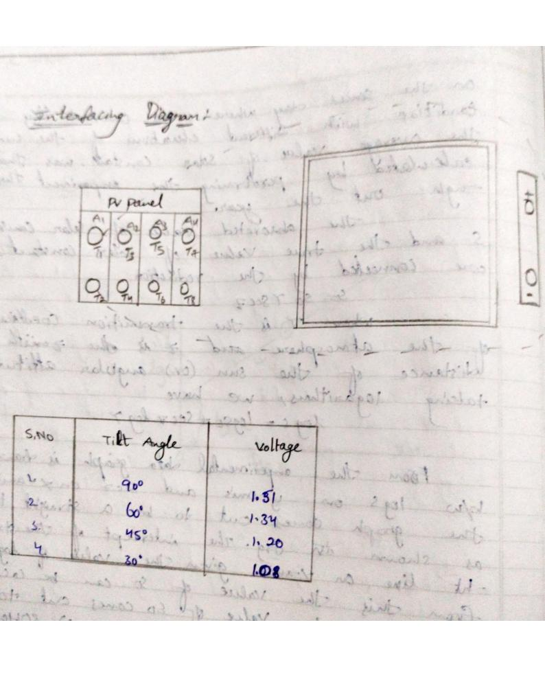
Date: 16/4/12 Page No. 5 Experiment No. 3 Photovoltic ponel sevies combination Experiment Name: Combination the photovoltic pound is server Requirement? 1. Solar panel trainer 2. Solar panel setup 3 patch chords prodedure! panel trainer using a pin cable.
