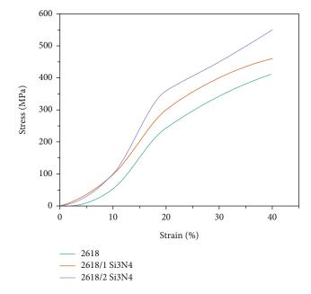
FIGURE 3: Curves of the samples' compression stress and strain.
