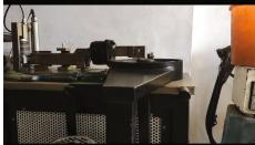
FIGURE 2: Pin on disc wear setup.
