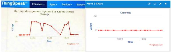
Real time voltage monitoring of battery
