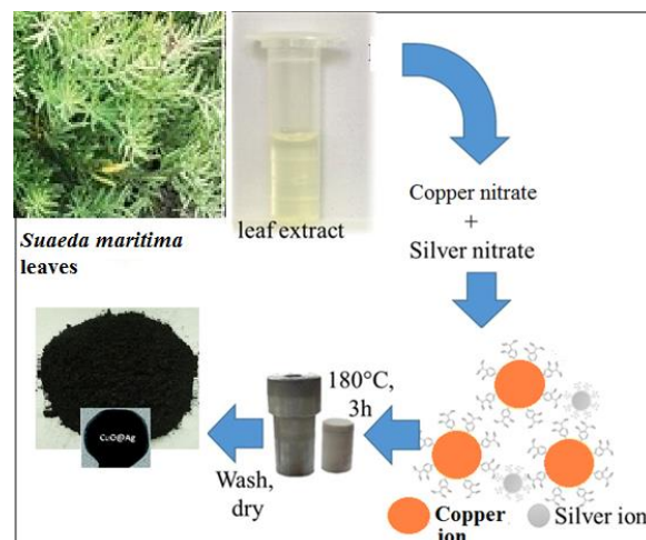
Figure 3: Preparation of Silver-copper oxide nano composites
